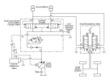
Figure 13 Dual Closed Center Brake Circuit in a Non-Dedicated Load Sense Hydraulic System
