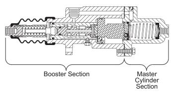
Figure 5 Open Center Power Brake Valve
