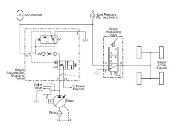
Figure 11 Single Closed Center Brake Circuit in a Non-Dedicated Open Center Hydraulic System
