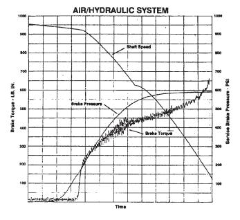
Figure 9 Time response - Air/hydraulic
