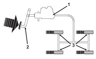
Figure 2 Simple Non-Boosted Brake System
