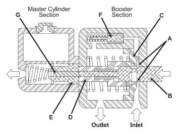
Figure 6 Two Fluid Power Brake Actuator
